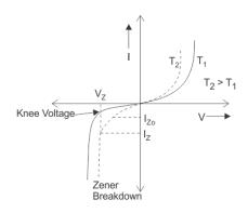
and distinct, the doping is controlled and the surface imperfections are avoided. In the V-I characteristics above Vz is the zener voltage, we can say. It is also the knee voltage because at this point the current is the current is very rapid.
